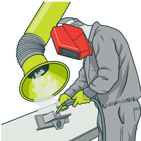
**FIGURE 5:** Flexible capturing hood
