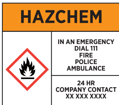
FIGURE 2: Sample sign for substances in a building (but not a dedicated room/compartment)
