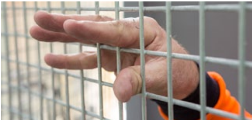
Figure 6: The reach is restricted by the roots of the fingers.
