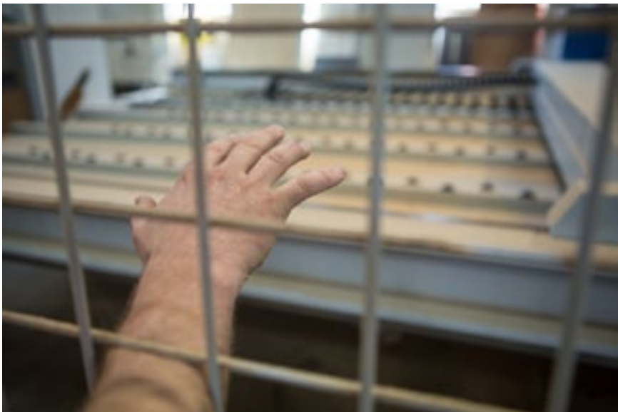
Figure 7: The distance of the guard from the dangerous part is worked out by how far someone can reach.
