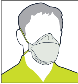
Disposable respirator (for low to medium dust levels)
