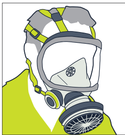
Full-face respirator (for medium dust levels)
