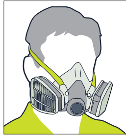
Half-face respirator (for low to medium dust levels)
