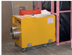
A negative pressure unit must be installed to remove air from within the enclosure
